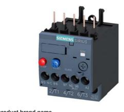
Overload relay 2.2...3.2 A Thermal For motor protection Size S00, Class 10 Contactor mounting Main circuit: Screw Auxiliary circuit: Screw Manual-Automatic-Reset
