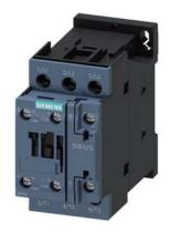
power contactor, AC-3 25 A, 11 kW / 400 V 1 NO + 1 NC, 230 V AC, 50 Hz, 3-pole, Size S0 screw terminal
